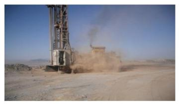
Fig. 2. Ingersoll-Rand T4BH Drill Rig in the mine
